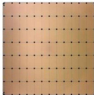
Cerebras WSE-3 4 Trillion Transistors 46,225 mm 2 Silicon
